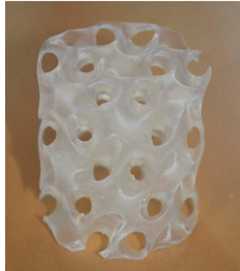
Figure 1: An example of a complicated shape that is easy to produce by 3D printing. Making a similar structure using traditional manufacturing methods would be difficult and time consuming.
